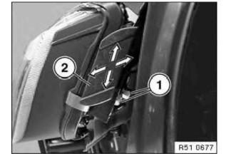
Unfasten nut (1) from wheel arch and remove bracket (2).
