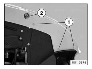
Loosen left/right hexagon bolts (1). Loosen left/right screw (2).
