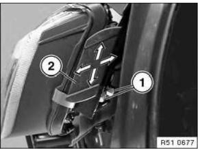
Loosen nut (1) from wheel arch and adjust bracket (2).
