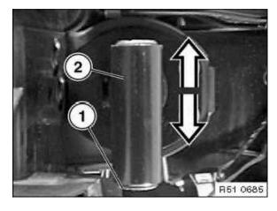
Height of bumper (in front area) is now adjusted by turning socket head cap screw (1) in shock absorber (2).
