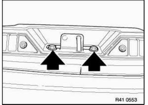
Loosen screws on lower section of trunk lid lock until it can just be moved, enabling it to center itself.
