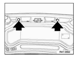
Screw in detent buffer until left and right sides of trunk lid locate against detent buffers when closed.
