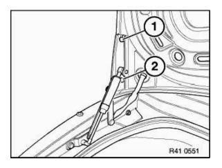
Loosen left and right bolts (1). Unscrew left and right bolts (2). Remove trunk lid.
