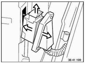
Unhinge door by moving upwards and placing it on a suitable surface.
