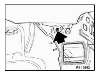
Unfasten screw for retainer on side panel of rear wheel arch. Remove rear side panel.
