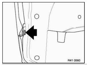
Unfasten screw for trim retainer on cover of side member and rear side panel.
