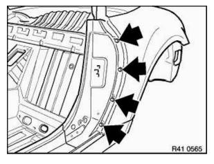
Retaining screws from rear side panel on B-pillar.
