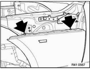
Unscrew upper mounting bolts. Remove front side panel.
