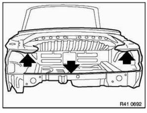
Remove scrap metal. Grind down and straighten mating surfaces.
