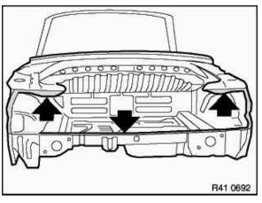
Coat connection points on the body with zinc dust paint.
