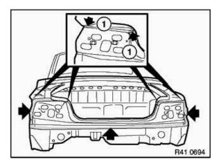
Adjust tail panel to fit, secure and weld up. Braze tail panel in these areas (1). Grind down connection points and seal.
