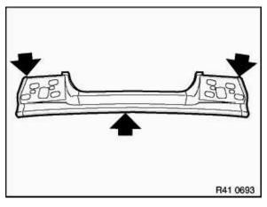
Clean connection point on spare tail panel and coat with zinc dust paint.
