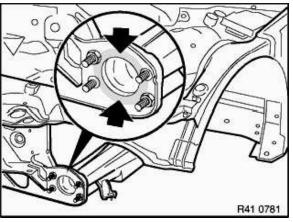
Drill off welding spots at left and right. Remove front wall.
