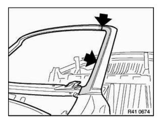
Expose and clean connection point between top of windshield and wind cowl panel.
