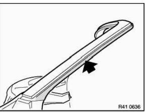
Weld connection point on outer windshield.
