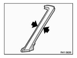
Clean connection points on spare part. Align and secure spare part.
