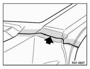
Weld connection point on lower windshield. Grind welding spots until they are smooth.
