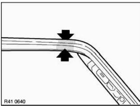
Tin out connection point on top of windshield and grind down.
