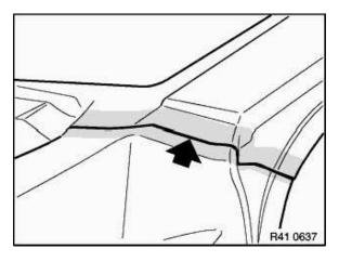
Expose connection point at bottom of windshield. Remove cowl panel.
