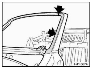
Weld spare part at top of connection point between windshield and cowl panel.
