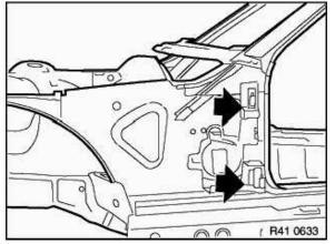
Remove scrap metal. Straighten and grind joint surfaces.
