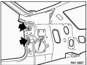
Weld door hinges from inside vehicle.
