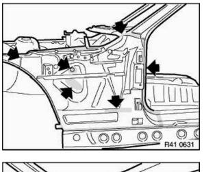
Adjust spare part to fit and secure. Weld spare part.
