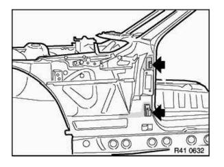
Roughly cut away cover for A-pillar around the door hinge. Remove A-pillar cover.
