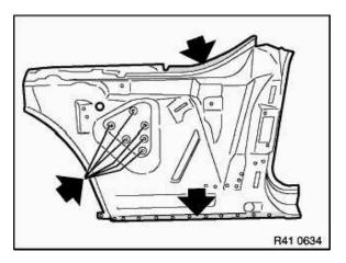
Drill holes for plug welding of spare A-pillar cover in the region of:
