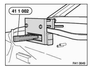
Insert punch numbers 41 1 002 individually in special tool 41 1 001 and emboss the chassis number.
