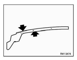
Apply an adhesive bead of original BMW windshield adhesive approx. 15 mm high within the marked contact surface of the shaped part.
