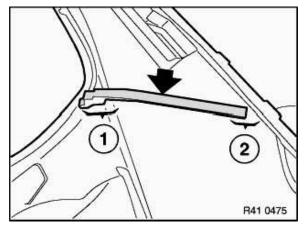
Apply an approx. 15 mm high bead of original BMW windshield adhesive on the contact surface of the shaped part.
