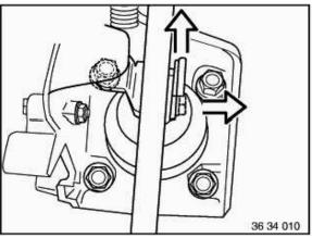
Remove panelling for instrument panel at bottom left, refer to Gr. 51
