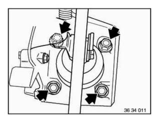
Unscrew nuts and remove brake booster
