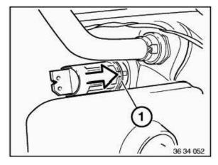
Mount new snap ring (1) in groove of sensor holder in brake booster.
