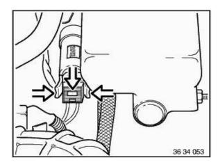
Lift snap ring out using a screwdriver.
