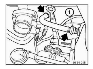
Disconnect vacuum hose on intake manifold and non-return valve (1).
