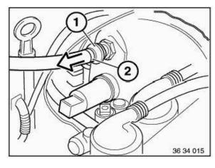
Loosen clamp (2) and pull out non-return valve (1).
