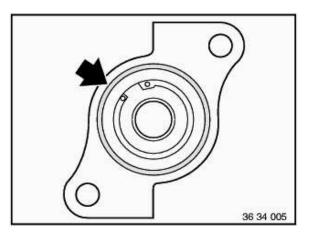
Use new seal between brake master cylinder (tandem) and brake booster.
