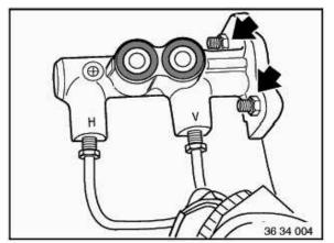
Unscrew lock nuts and pull brake master cylinder (tandem) out of brake booster.
