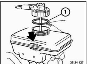
Correct brake-fluid level. Check seal (1).
