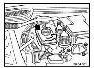
Draw brake fluid out of the expansion tank with a suction bottle, which may only come into contact with brake fluid.
