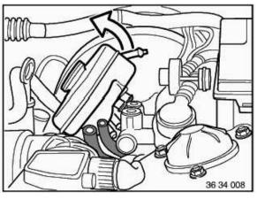
Disconnect expansion tank from brake master cylinder (tandem) by tilting to side.
