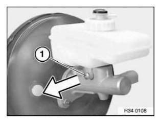
Loosen mounting bolt (1) and pull out completely.
