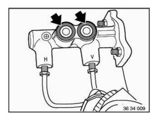
Coat sealing rings only with brake fluid. Do not use ATE brake-cylinder paste.
