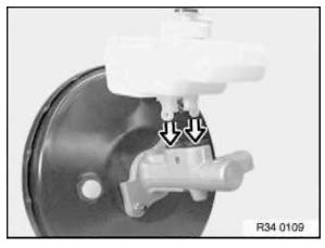
Press tank into plugs with connectors as far as stop so that they are precisely perpendicular.
