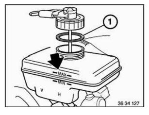
Fill expansion tank with new brake fluid until level reaches MAX mark (refer to specifications on BMW Operating Fluids).
