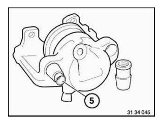
Check guide sleeves (5), installing guide sleeves from repair kit if necessary.
