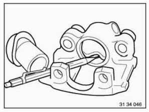
Remove sealing ring carefully with a plastic needle.
