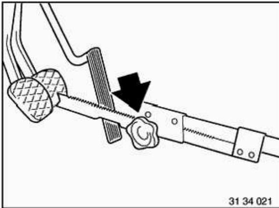
Apply pedal prop and depress brake pedal slightly. This prevents brake fluid from escaping from expansion tank after brake pipes have been disconnected (which would enable air to enter the braking system).
