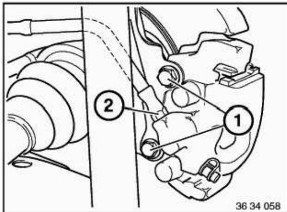
Loosen screws (1). Disconnect brake hose (2).
