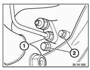
Unscrew brake pipe (1) and plug with a rubber cap or nipple. Unscrew bolts (2) and remove wheel-brake cylinder.
