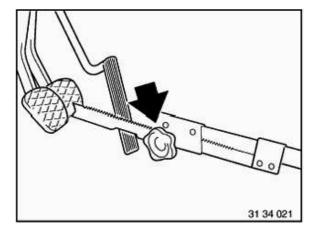
Apply pedal prop and depress brake pedal slightly. This prevents brake fluid from escaping from expansion tank after brake pipes have been disconnected (which would enable air to enter the braking system).
