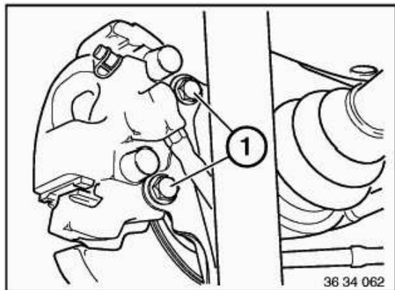
Unscrew bolts (1). Remove and suspend brake caliper from vehicle.
