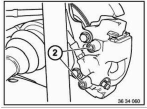
Unfasten guide screws (2) with special tool 34 1 040 and pull brake caliper backwards to remove.
