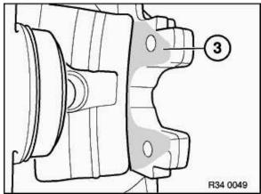
Clean contact surfaces (3) of brake linings on brake caliper and thinly coat with anti-squeak compound.
