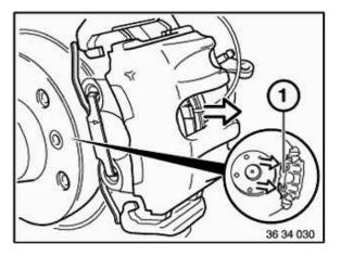
Lift out retaining spring (1).
