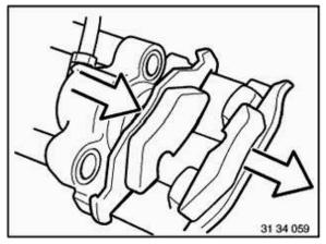
Remove outer brake lining.
