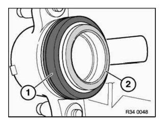
Check dust sleeve (1) for damage and replace if necessary. Clean contact surfaces (2) of brake piston and coat with a thin layer of anti-squeak compound.
