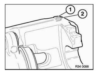
Clean contact surfaces (1 - 2) of the brake-lining tee heads on the brake caliper and thinly coat with anti-squeak compound. Anti-squeak compound, refer to BMW Service Operating Fluids.
