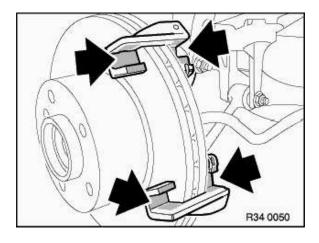
Clean hammerhead guides on brake caliper holders and apply thin coat of anti-squeak compound.
