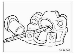
Remove sealing ring carefully with a plastic needle. Clean cylinder bores and parts with alcohol and dry with compressed air.
