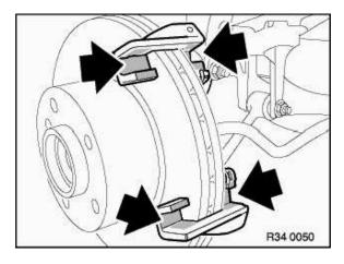
Clean hammer head guides on brake caliper holders and coat with a thin layer of anti-squeak compound.
