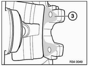
Clean contact surface (3) of brake linings on brake caliper and thinly coat with anti-squeak compound.
