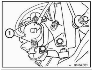
Unfasten guide screws (1) and lift out brake caliper towards rear of vehicle.
