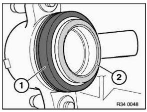
Check dust sleeve (1) for damage and replace if necessary.
