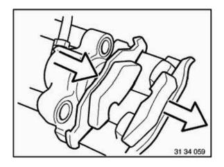
Remove outer brake lining.
