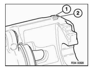
Clean contact surfaces (1 - 2) of brake-lining tee heads on brake caliper and thinly coat with anti-squeak compound. Anti-squeak compound, refer to BMW Service Operating Fluids.
