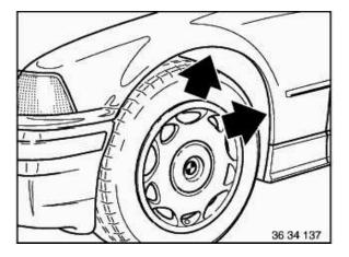
5. Bleed accumulator ASC+T (only vehicles up to 09.93) Remove liner from inside of front-left wheel house.
