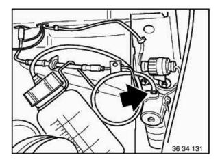
Connect bleeder hose with bottle to bleeder valve (accumulator).
