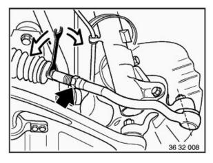
Loosen lock nut on track rod.
