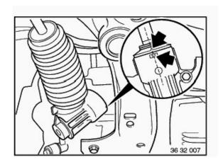
Adjust toe and toe-difference angle.
