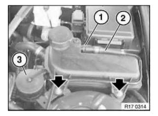
Release clamp (1) and detach vent hose (2) from coolant expansion tank.
