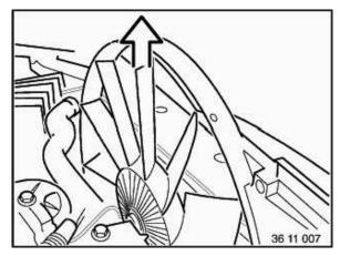
Lift out fan cowl and fan impeller together.
