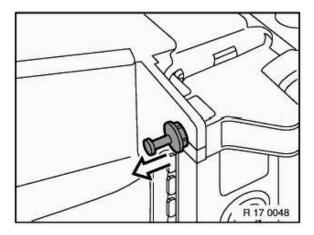
Lever out expansion rivets on left and right from fan cowl.
