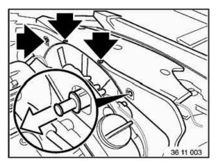
Lever out expansion rivets and pull out air duct on left and right.
