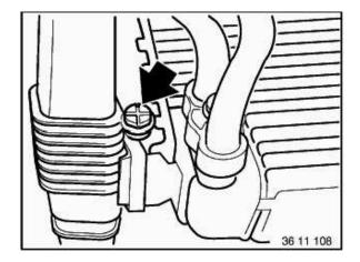
Remove front underbody protection and unfasten drain plug at bottom of radiator if necessary.
