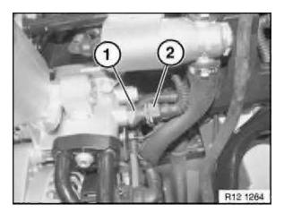
Unlock plug (1) and detach from oil pressure switch (2). Unscrew oil pressure switch (1). Tightening torque, 12 61 1AZ..
