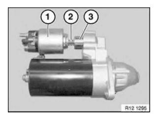
Remove solenoid switch (1) and spring (2). Unhook pin (3).
