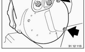
Check collector ring for wear and recondition if necessary.
