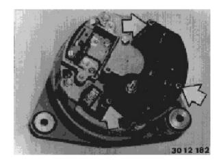
Unsolder stator winding on diode plate
