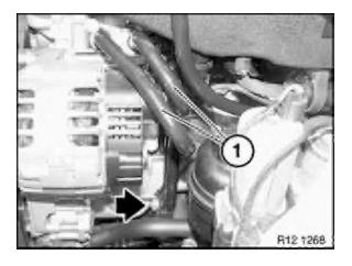
Release screw on holder for oil cooler lines (1).
