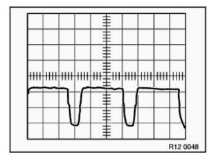
Open circuit in exciter diode. Repair/exchange alternator.
