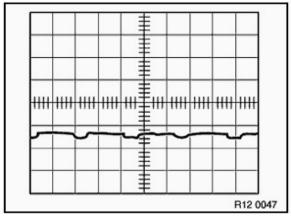
Short circuit in positive diode. Repair/exchange alternator.
