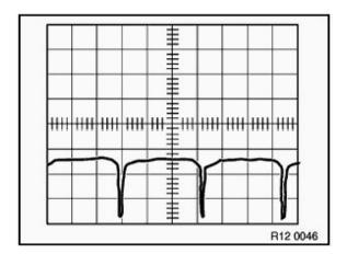
Open circuit in negative diode. Repair/exchange alternator.
