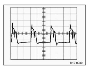
Open circuit in positive diode. Repair/exchange alternator.
