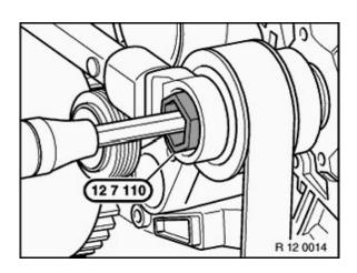
Remove and install alternator drive belt.
