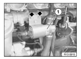
Release nuts and place idle-speed control valve (1) to one side.
