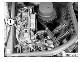
Unlock plug (1) and detach from DME control unit. Remove DME control unit.
