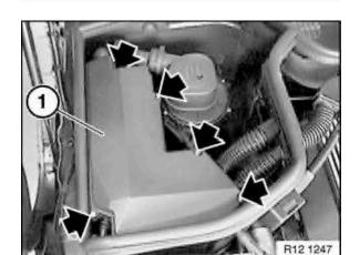
Release screw connection of electronics box (1). Remove electronics box (1).
