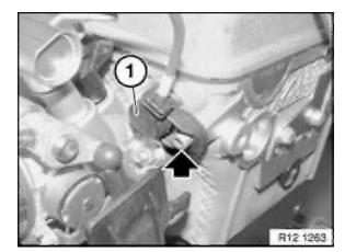
Release screw on pulse generator (1).
