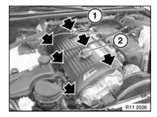
Unlock plug lock (1) for ignition coil.
