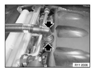
Press locks. Remove hose for engine vent.
