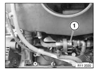
Detach tank venting valve (1) from holder on manifold.
