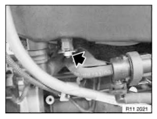
Detach manifold support at front and rear from intake air manifold.
