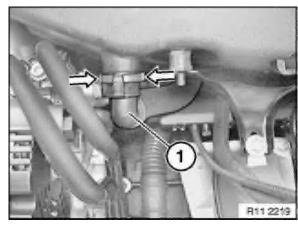
11 9 160 E11 2126 Press lock. Detach hose (1) from intake air manifold.
