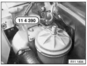
Insert special tool 11 4 390 and tighten down oil filter cover.
