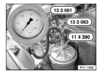
Connect special tools 13 3 061 / 063. Start engine and check engine oil pressure.
