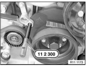
Remove special tool 11 2 300. Adjust valves. Assemble engine.
