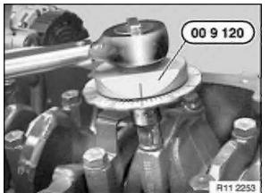
Secure conrod with special tool 00 9 120. Tightening torque:
