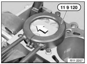
Keep piston rings pressed with special tool 11 9 120. Install piston so that arrow points to camshaft drive.
