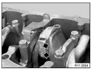
Apply light coat of oil to connecting-rod bearing shells. Fit bearing caps so that pair numbers match up.
