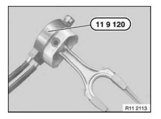
Lightly coat pistons and piston rings with oil.
