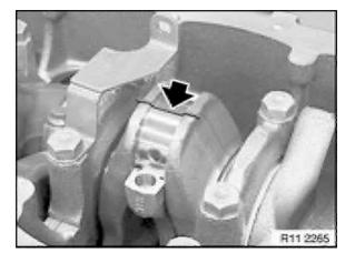
Check connecting-rod bearing clearance:
