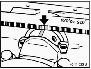
Remove bearing cap and read off bearing play at width of flattened plastic thread with assistance of measurement scale.
