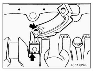
Insert main bearing caps in such a way that guide grooves of main bearing shells lie on one side.
