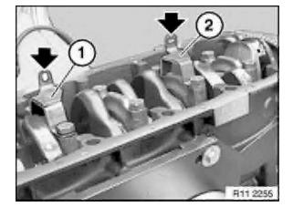
Holders for oil lines are fitted on main bearing caps 3 and 5.
