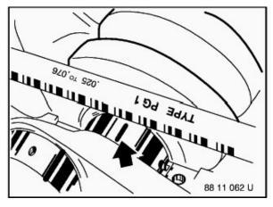
Remove main bearing cap and read off bearing clearance at width of pinched plastic thread on measuring scale.
