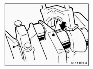
Check clearance on main crankshaft bearing.
