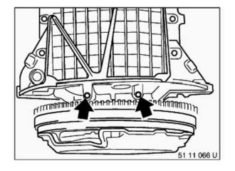
Release screws in end cover at rear.
