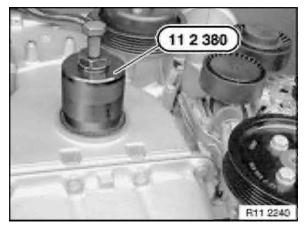
Screw in special tool 11 2 380 until it is firmly connected to the radial seal.
